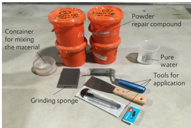
Photo: Equipment and working aids
